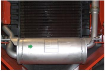
The diesel particle filter is integrated in the original silencer. All existing connections remain available in their original condition.
