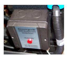
The pressure monitoring unit is installed in the drivers cabin and is good visible.
