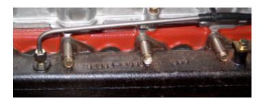
The back pressure pipe has to get screwed on to the manifold with an 1/8" thread. The Teflon line is connected from the back pressure pipe to the control device. The control device is installed in the engine compartment.
