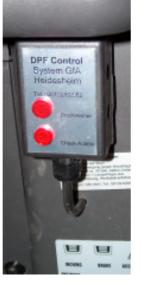
The pressure monitoring and the control unit in the drivers cabin is good visible.
